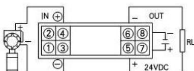
④配电电源正极、③配电电源负极
